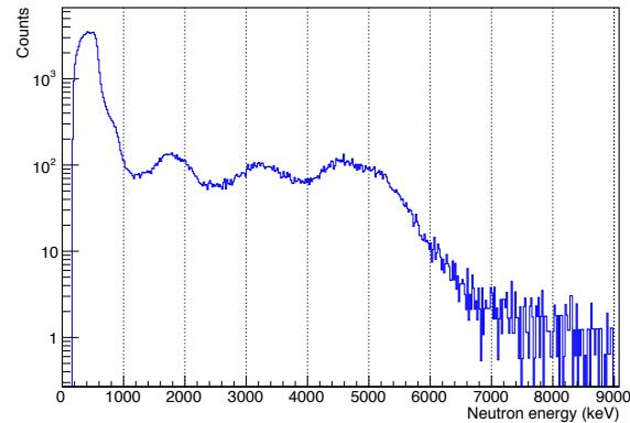
Measured neutron spectrum at 60 deg
