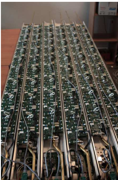
Detector installed in a 70T/h sorting machine
