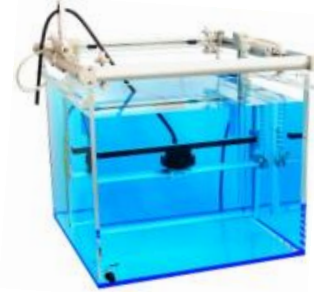
5 th gen. water phantom Blue Phantom®
